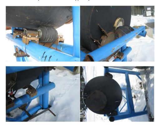
Compost is added to the barrel through the top door. The whole composter is rotated about once a week. The barrel is shown as full and will be locked closed to work for the first five weeks of warm weather. The second system should be in place in May.
