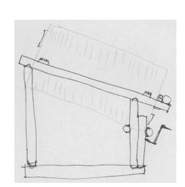
The end of the barrel was cut away, cleaned, a baffle set in place, and teeth about 12 inches long set around the inside of the barrel. A door was set in both ends of the barrel. The doors are hinged and overlap an internal ring.
